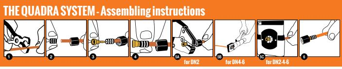
Cut the QUADRA capillary hose to the required lenght using the special WXAOO4 cutter Slip the nut over the hose (depending on fi tting type). Ensure that the threaded side is pointing towards the end of the hose that needs assembling. Henden to the hose that hose end y assembling.
